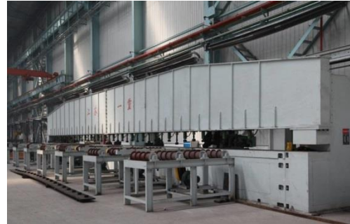
18-m Planing & Milling Machine Processing Thickness 6-150mm Processing width 500-1100mm 18000mm
