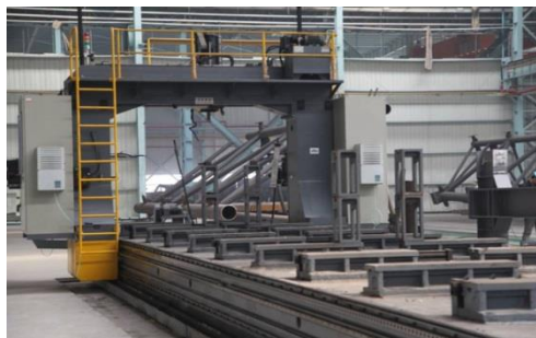
Gantry Movable NC 3D Drilling Machine processing width 1000-2000mm
