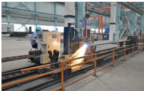
NC Intersecting line Cutting Machine Machining diameter 60-800mm
